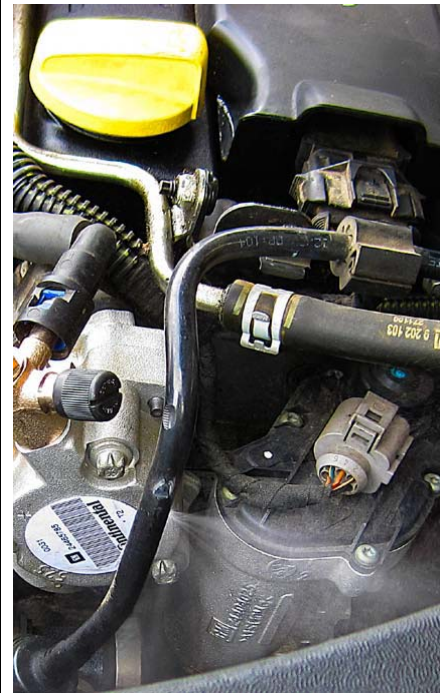
The pump (silver device) leaks: externally, the damage is invisible
